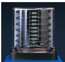
Anesthesia machine bellows. The excursion of the bellows indicates the tidal volume.
